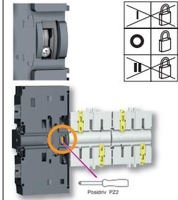
⚠ To allow padlocking in all positions (I - 0 - II), configure the ATyS M as follows before installation. (Screw is located at the back of the product).
