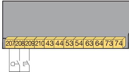
Following an emergency trip, the fault must be validated and inhibited to allow the resumption of automatic operation (by opening then closing the Auto-Man cover, activating the RST input or via the RS485).
