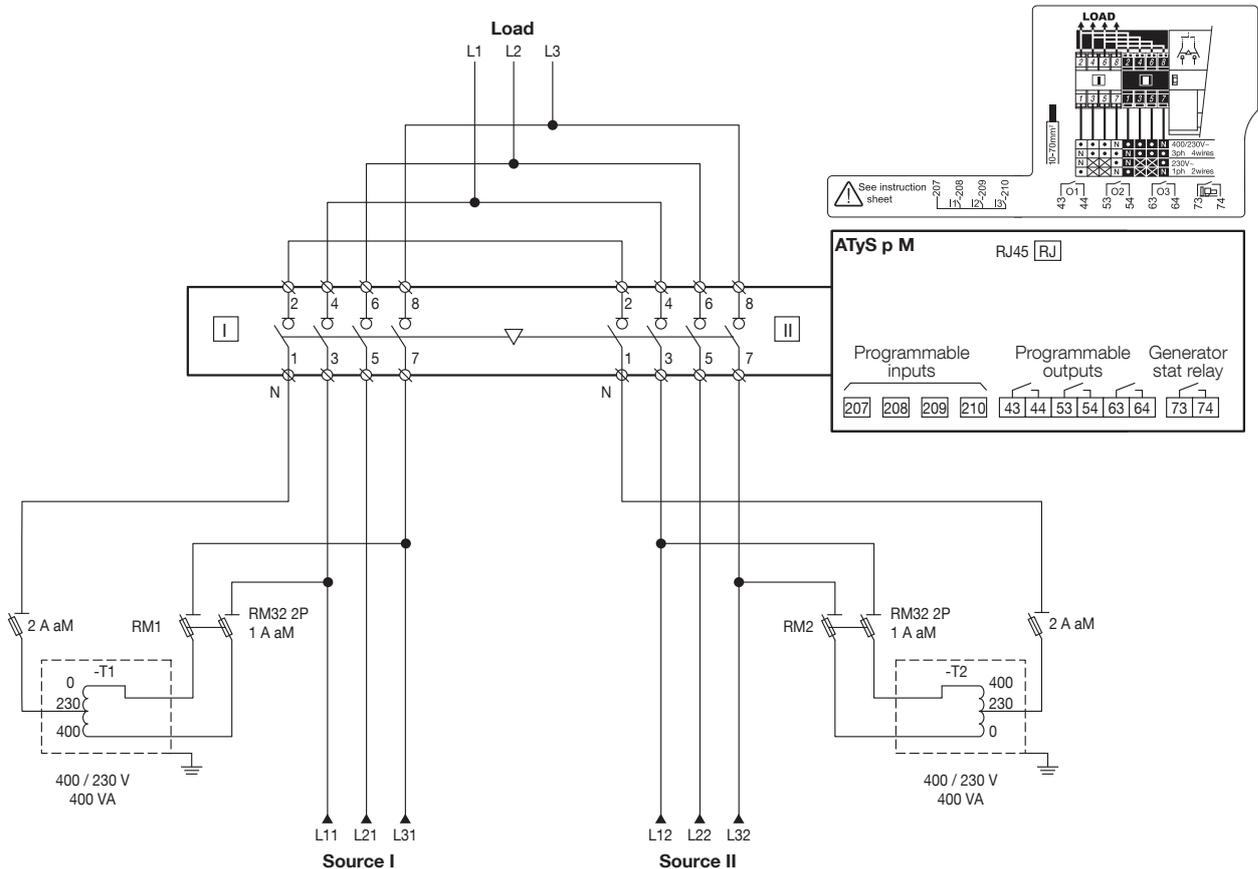
In case of use with an auto-transformer, the following wirings have to be respected in order to maintain the control of the rotation functionality:
