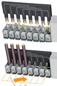
Voltage taps provide 2x ≤ 1.5mm<sup>2</sup> connections. They can be fitted in any terminals on the source supply side. Do not use on the load side when equipped with a bridging bar.
