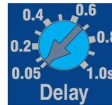
The adjustment for "Delay (s)" sets the period that the P9620 waits before the relay energises once the "Low-set" threshold "lo>" has been exceeded.
