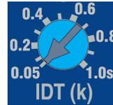
The adjustment for "IDT (k)" (Time Multiplier) defines the tripping characteristic when the "Low-set" threshold "I>" has been exceeded. The lower the setting, the faster the response to tripping. The higher the setting, the slower the response.
