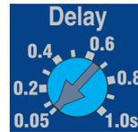
The adjustment for "Delay" defines the delay period between exceeding a trip threshold on any of the phases and the relay energising.
