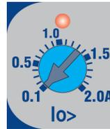
The adjustment for the "Low-set" can be set from 0.1 to 2A. When the threshold is exceeded due to an Earth fault condition, the corresponding red LED above the adjustment illuminates indicating activity. When tripping finally occurs, the red LED will then flash.
