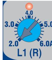
Individual adjustments for the trip threshold allow the user to set each phase independently of each other. When the threshold is exceeded on any phase due to an Overcurrent condition, the corresponding red LED above the adjustment illuminates indicating activity. When tripping finally occurs, the red "Trip" LED will then flash.
