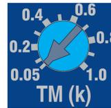
The adjustment for "TM (k)" (Time Multiplier) defines the tripping characteristic when the "Low-set" threshold "lo>" has been exceeded. The lower the setting, the faster the response to tripping. The higher the setting, the slower the response.
