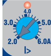
The adjustment for the "Low-set" can be set from 2 to 6A. When the threshold is exceeded due to an Overcurrent condition, the corresponding red LED above the adjustment illuminates indicating activity. When tripping finally occurs, the red LED will then flash.
